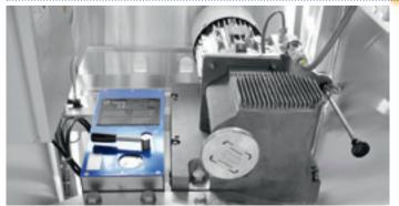
The heart of the G-servicelift is the G-trac and the G-lock® from goracon. Available in the categories of 400 kg up to 1100 kg for personal conveyance, the G-trac® and G-lock® are truly outstanding in terms of "Made in Germany "quality. The reliable and easy-to-use features of this hoist for personal conveyance, combined with the precise trigger mechanism of the fall arrest device, ensure that your personnel will be conveyed safely upwards in the **G**-servicelift°.
