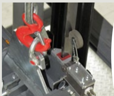
5 End of suspension rope secured to cabin carrier
